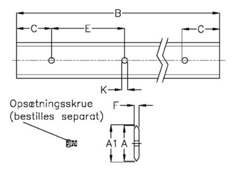
For bearing = 54For screw = M10x25 K = 11.5 Weight kg/1000 = 5000
